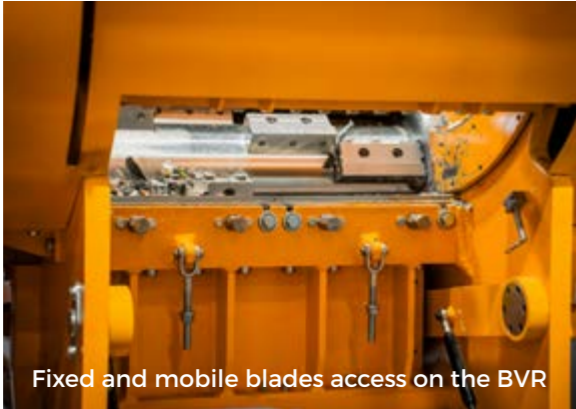
Screen and fixed blades access on the
