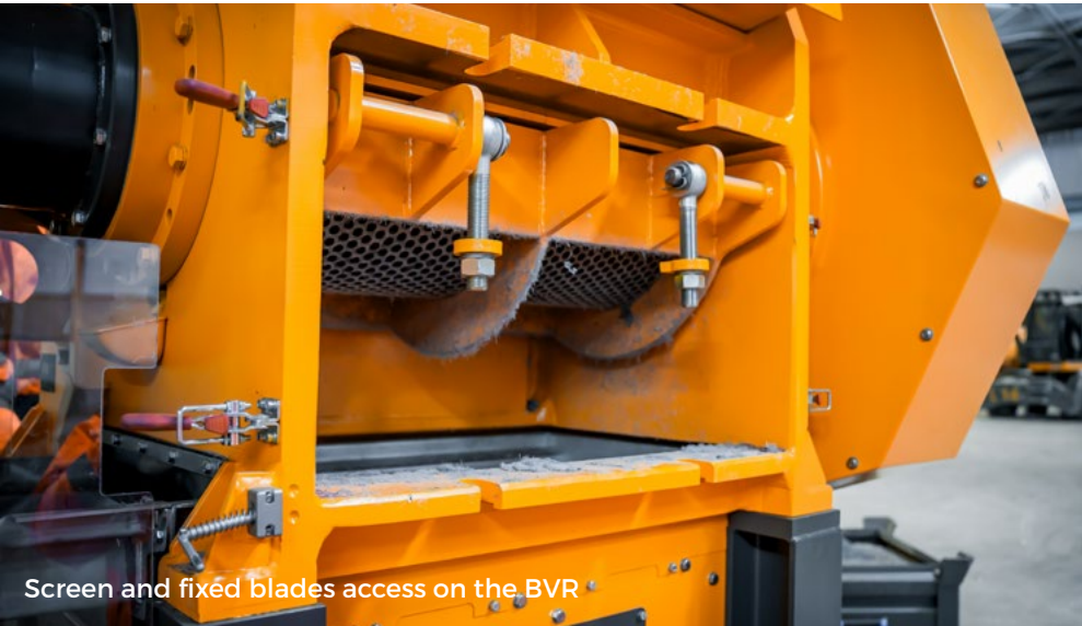
Screen and fixed blades access on the BVR
