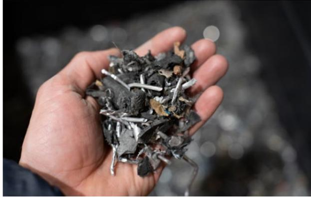
*Sample of crushed aluminum cable*
