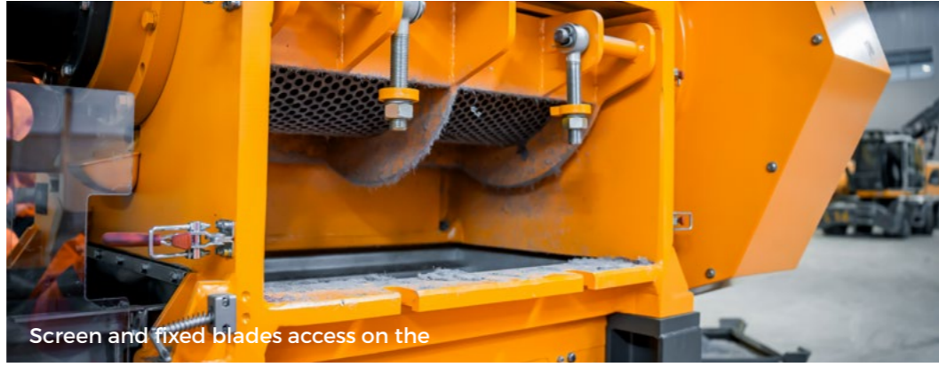
Fixed and mobile blades access on the BVR
